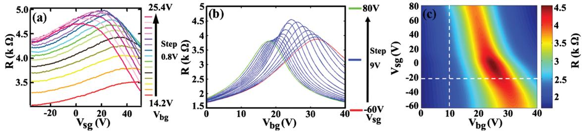
FIG. 2. (Color) (a) Resistance ( $R$ ) of the graphene device as a function of side gate voltage ( $V_{sg}$ ) at various back gate voltages ( $V_{bg}$ ). (b)  $R$  as a function of  $V_{bg}$  at various  $V_{sg}$ . (c) 2D color plot of  $R$  as a function of  $V_{bg}$  and  $V_{sg}$ . Curves in (a) and (b) correspond to vertical and horizontal line cuts in the color plot. All data measured in device “1” using SG1 as the side gate (Fig. 1).
